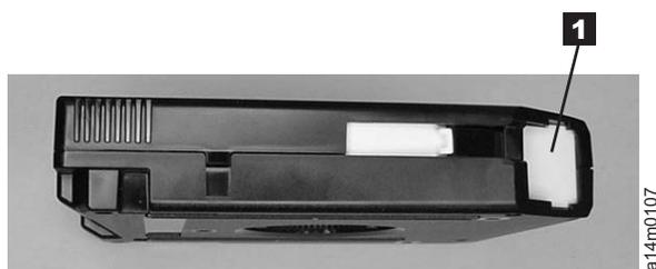
Figure 11. Cleaning cartridge door
