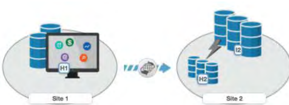
Figure 15. Global Mirror Failover/Failback with Practice session for FlashSystems/IBM Spectrum Virtualize and SAN Volume Controller
