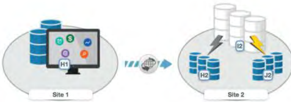
Figure 14. Global Mirror Failover/Failback with Practice session for DS8000 storage systems
