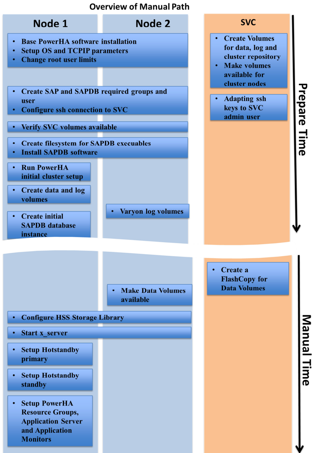
Figure 19 shows the sequence of steps which need to be taken for a manual installation. The sequence is not mandatory but represents a logical flow. The actual sequence will depend on the starting point, whether this is a new installation or a conversion.
