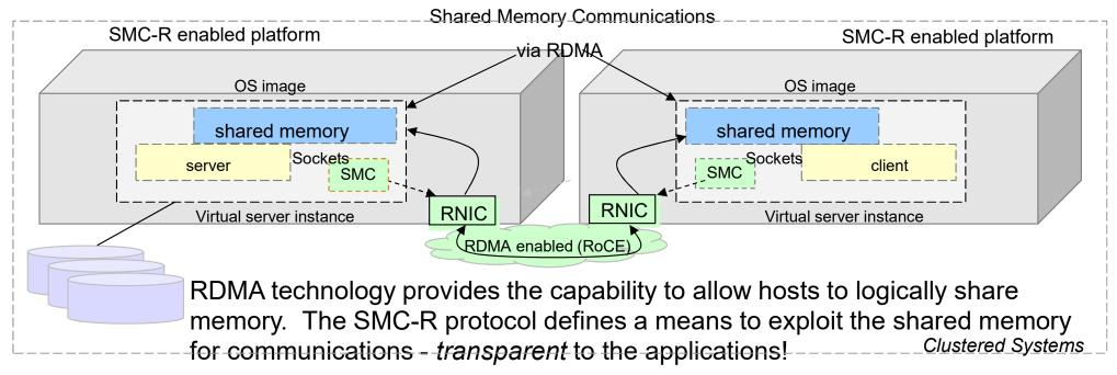
Shared Memory Communications – Remote (SMC-R) is an *open* sockets over Remote Direct Memory Access (RDMA) protocol that provides transparent exploitation of RDMA (for TCP based applications) while preserving key functions and qualities of service from the TCP/IP ecosystem that enterprise level servers/network depend on! SMC-R uses RDMA over Converged Ethernet (RoCE).
