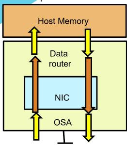
Latest OSAs use Direct Memory Access (DMA) and hardware data router, allowing data to flow through OSA without slower store and forward process.
