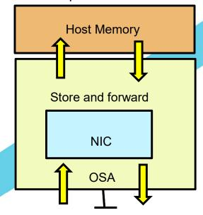
OSD and System Z can access shared memory. OSA interrupts the system using Peripheral Component Interconnect (PCI). The system interrupts OSA via Signal Adapter (SIGA) Instruction.
