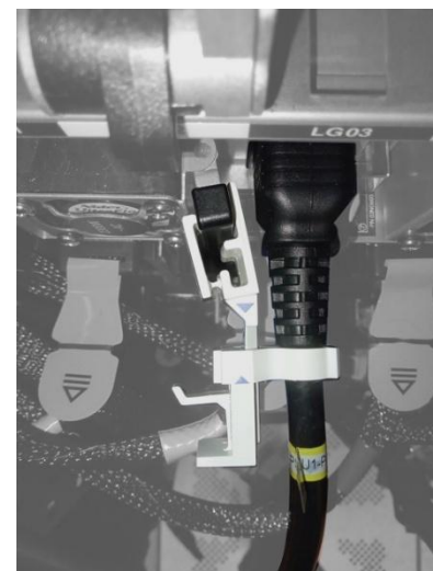
Figure 18: Large PSU Clip Fully Installed
