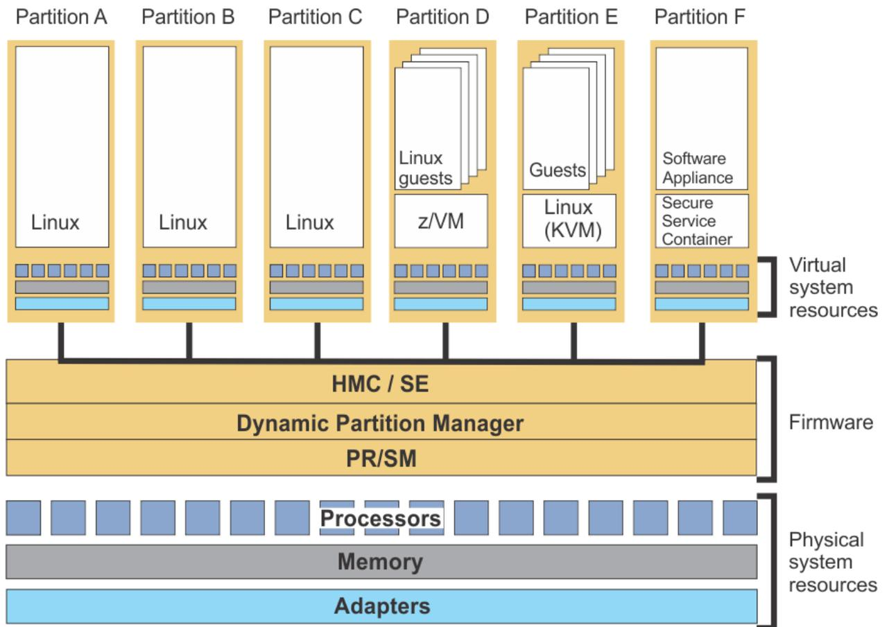
Figure 7. Partitions configured on a DPM-enabled system
