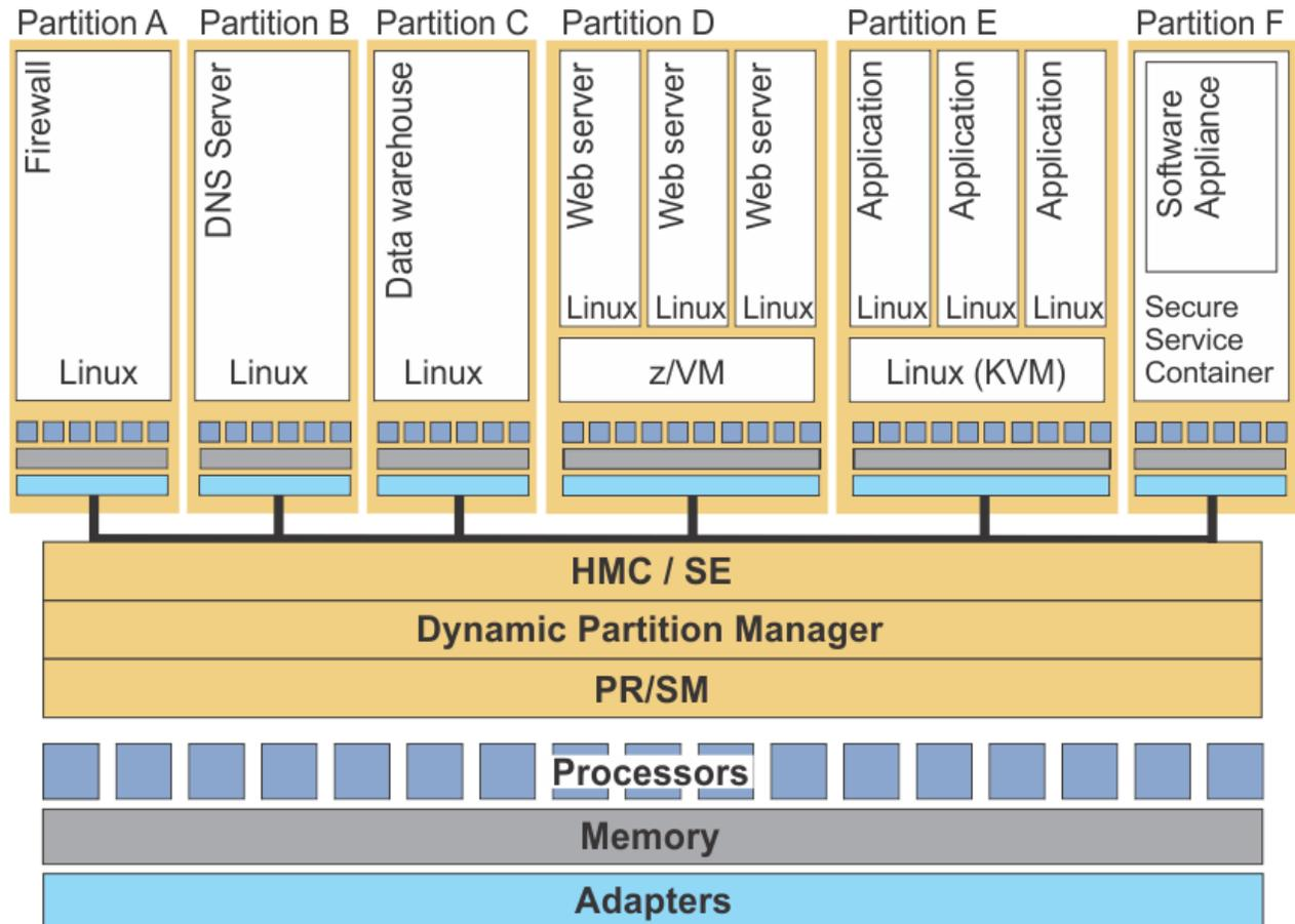
Figure 11. Example: Linux servers configured in partitions on a DPM-enabled system
