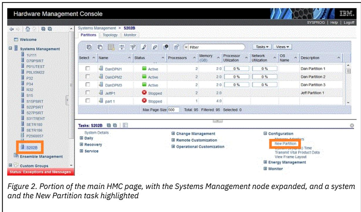
Figure 2. Portion of the main HMC page, with the Systems Management node expanded, and a system and the New Partition task highlighted
