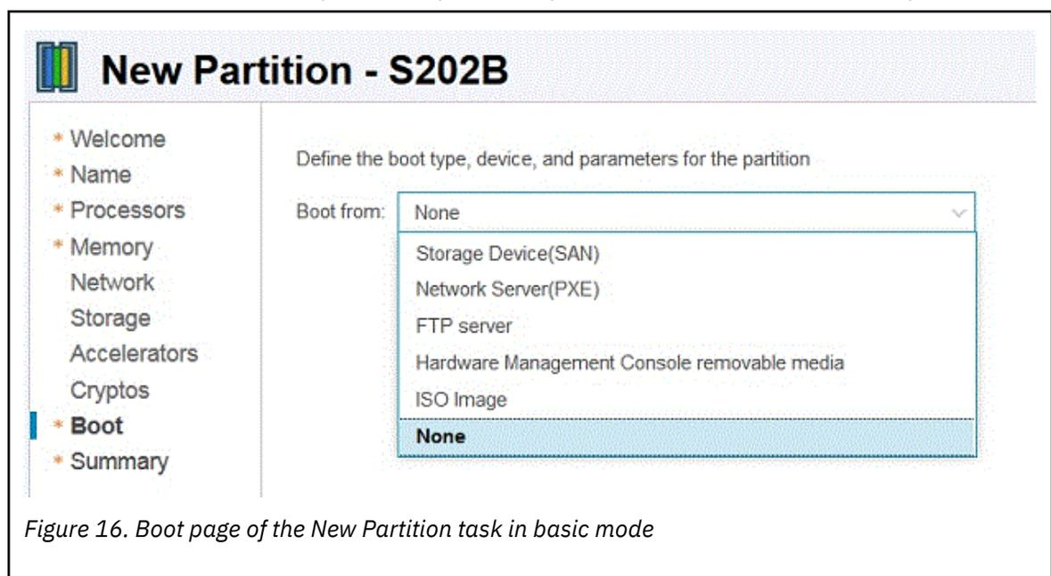
Figure 16. Boot page of the New Partition task in basic mode
