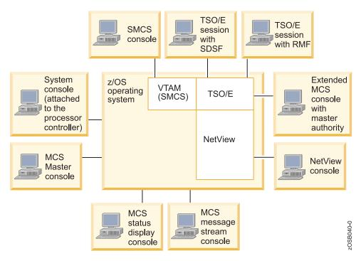
Figure 5. Sample console configuration for a z/OS system
