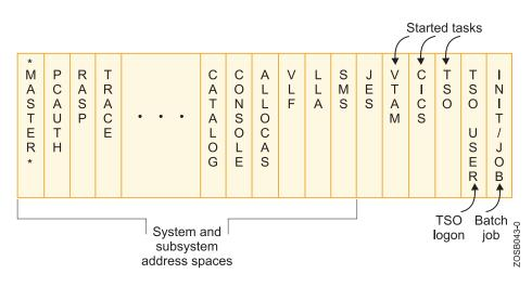
Figure 9. Virtual storage layout for multiple address spaces
