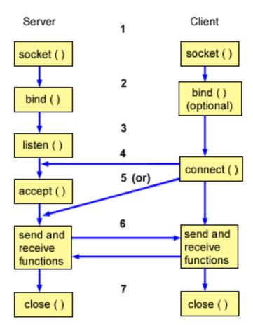
This is a typical flow of events for a connection-oriented socket:
