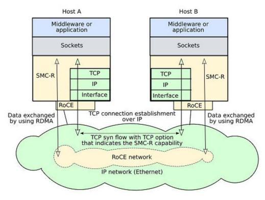
The SMC-R protocol solution is a hybrid solution that can be characterized as follows:
