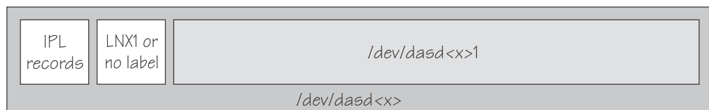
Figure 26. Linux disk layout
