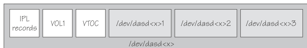
Figure 25. Compatible disk layout
