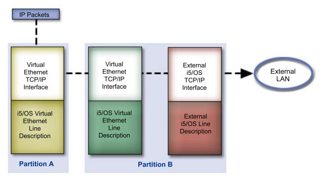
IP traffic initiated by partition A goes from its own virtual Ethernet interface to the virtual Ethernet interface on partition B. By implementing TCP/IP techniques used to connect virtual Ethernet to external LANs, you can enable the IP packets to continue on to the external interface and toward their destination.
