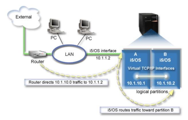
The existing TCP/IP interface (10.1.1.2) connects to the LAN. The LAN is connected to remote networks with a router. The virtual TCP/IP interface on partition B is addressed as 10.1.10.2 and the virtual TCP/IP interface on partition A as 10.1.10.1. In IBM i, if you turn on IP datagram forwarding, IBM i will route the IP packets to and from partition B. When you define your TCP/IP connection for partition B, the router address must be 10.1.10.1.
