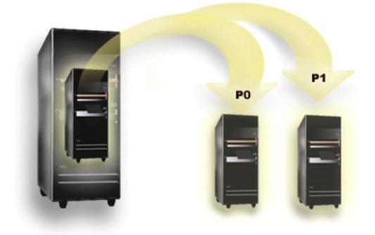
Logical partitioning is the ability to make a system run as if it were two or more independent systems. Each logical partition operates as an independent logical server. However, each partition shares a few physical system attributes such as the system serial number, system model, and processor feature code. All other system attributes may vary among partitions.
