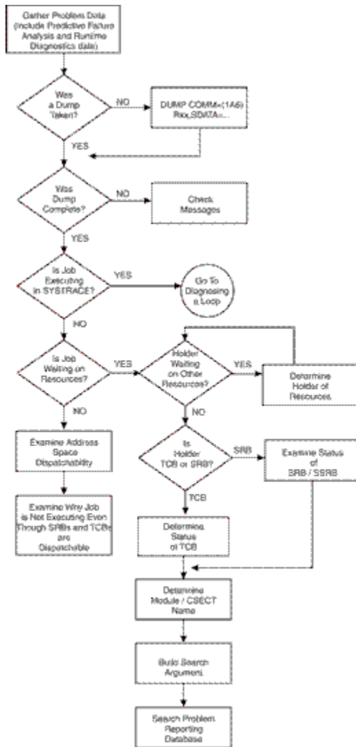
Figure 56. Flowchart for job or subsystem hang analysis
