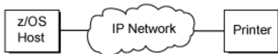
Figure 28. Appearance of the TCP/IP connection between a z/OS host and a printer
