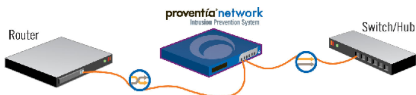
Figure 3: Router to switch or hub
