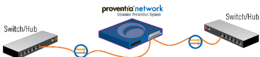
Figure 4: Switch or hub 1 to switch or hub 2
