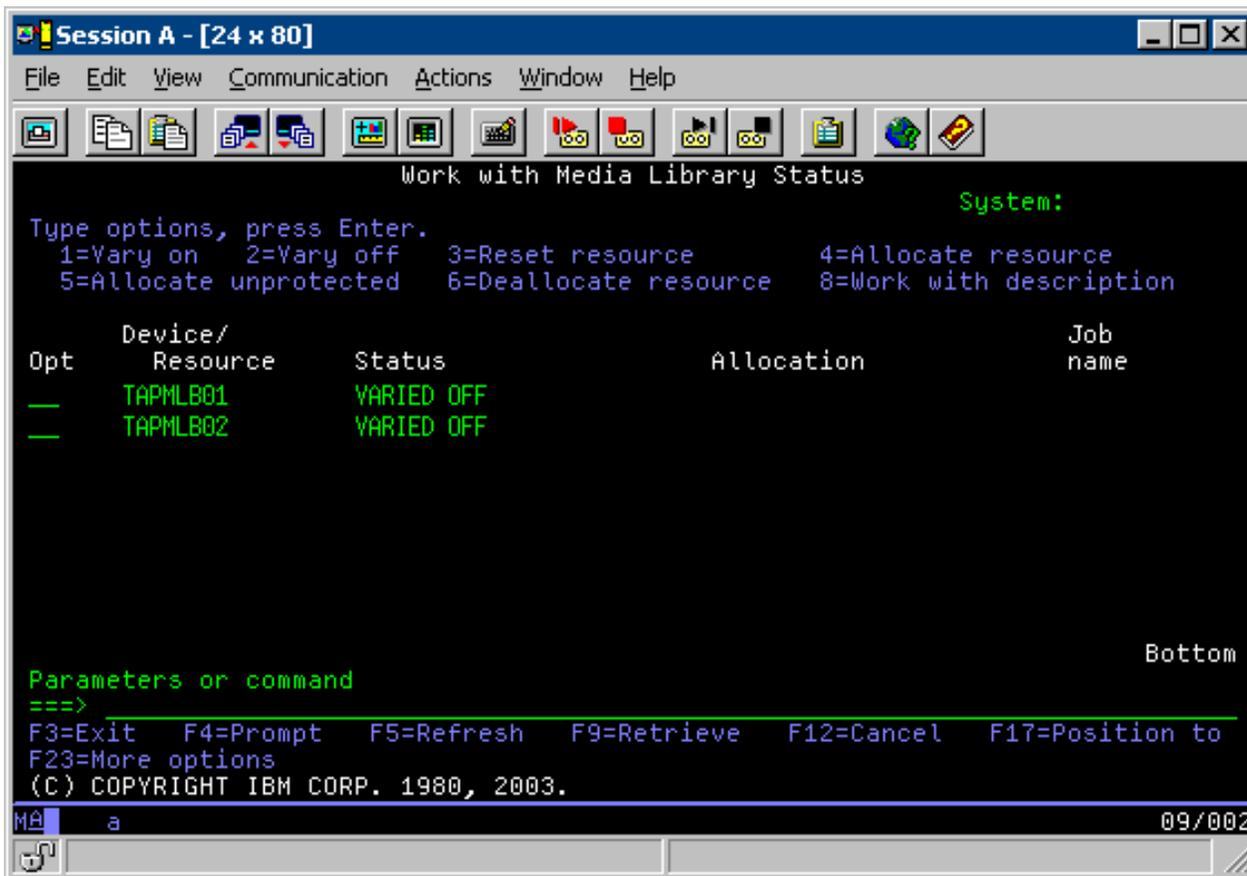
After the command CFGDEVMLB(TAPMLB01) is completed, you can see both resources under TAPMLB01, even though TAP02 actually generated TAPMLB02. Both resources are set to UNPROTECTED.
