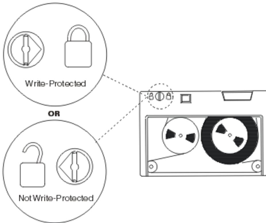
Figure 9. Write-protect positions for a newer-style quarter-inch tape cartridge
