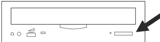
No preventive maintenance is necessary for the optical drive. Always handle optical disks by the edges to avoid finger prints. Optical disks can be wiped with a soft lint-free cloth or lens tissue. Always wipe in a straight line from the inner hub to the outer rim.
