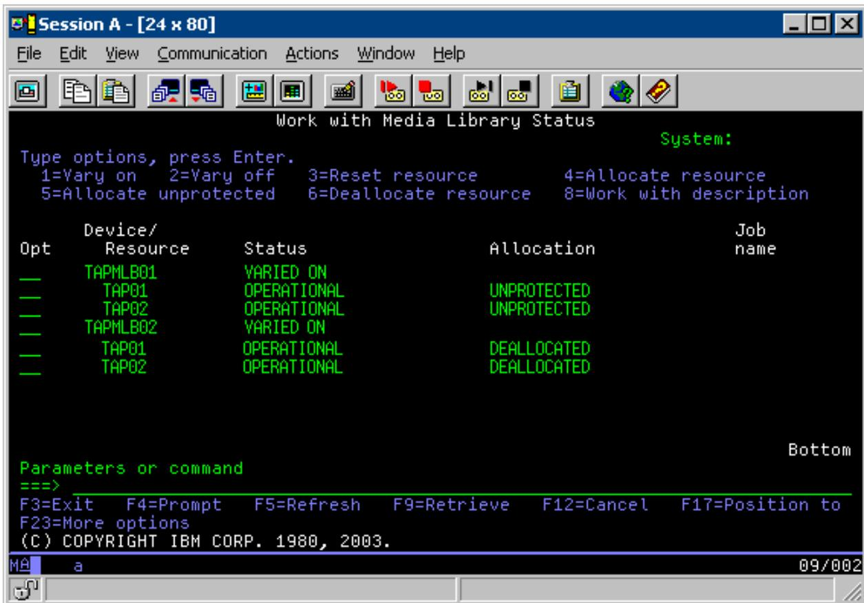
In order to use the TAPMLB02 device description, you set TAP01 to UNPROTECTED in TAPMLB01 and you set TAP02 to UNPROTECTED in TAPMLB02, as is shown in the following display.
