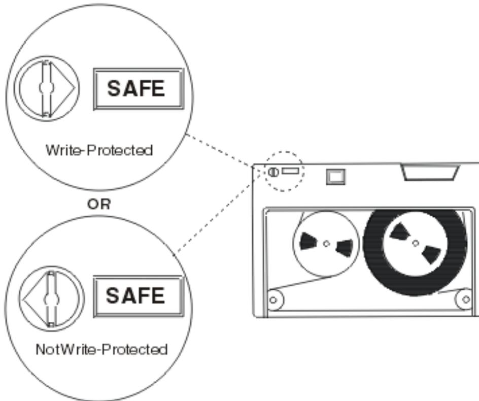
Figure 8. Write-protect positions for an older-style tape cartridge
