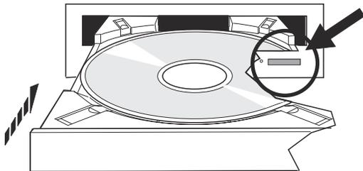
4. To remove the disk from the drive, look at the following figure and press the Eject button.
