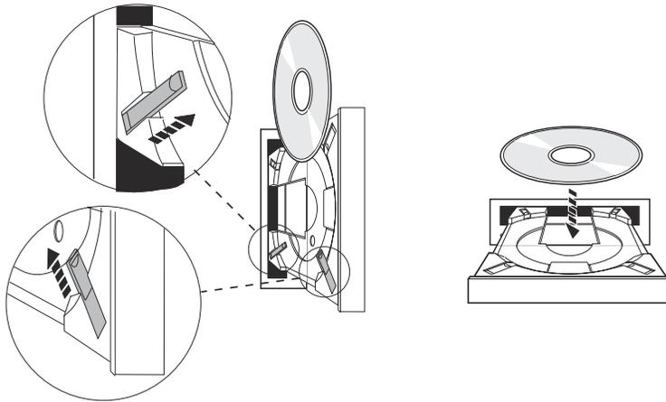
3. When you have properly positioned the disk in the tray, press the Eject button or push the tray into the drive as shown in the following figure.
