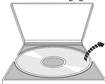
2. Slide the disk into the tray with the label side showing. If your optical device is vertically positioned, make sure that the disk is secured by the two tabs at the bottom of the tray as shown on the left in the following figure.
