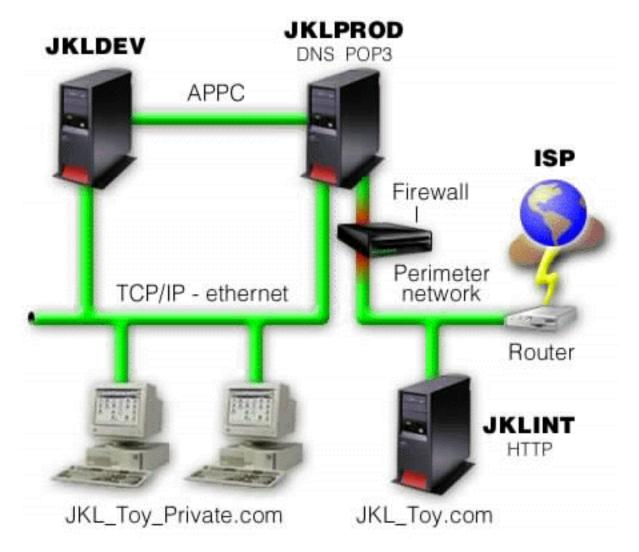
As shown in the figure, JKL Toy Company has two primary systems. They use one system for development applications (JKLDEV) and one for production applications (JKLPROD). Both of these systems handle mission-critical data and applications. Consequently, they are not comfortable running their Internet applications on these systems. They have chosen to add a new system (JKLINT) to run these applications.
