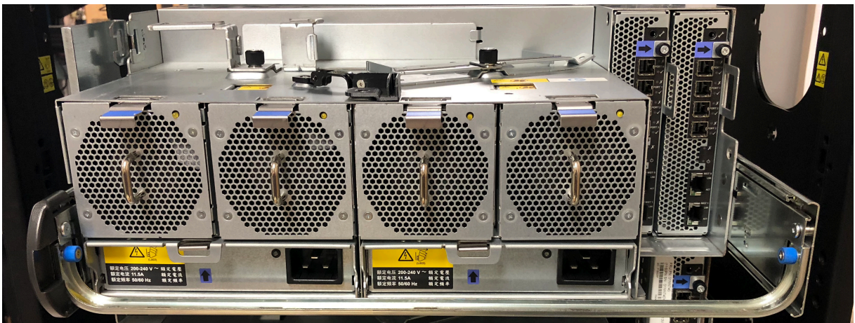
Figure 49. Crossbar with blue thumbscrews stabilizes the two rails at the rear of the chassis
