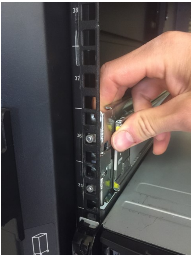
Figure 34. Front rack post attachment details
