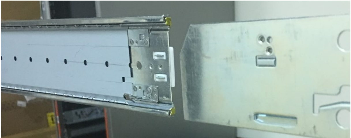
Figure 40. Rail slide alignment detail
