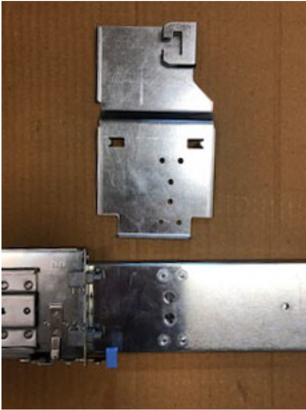
Figure 28. CMA attachment aligned with outer slide
