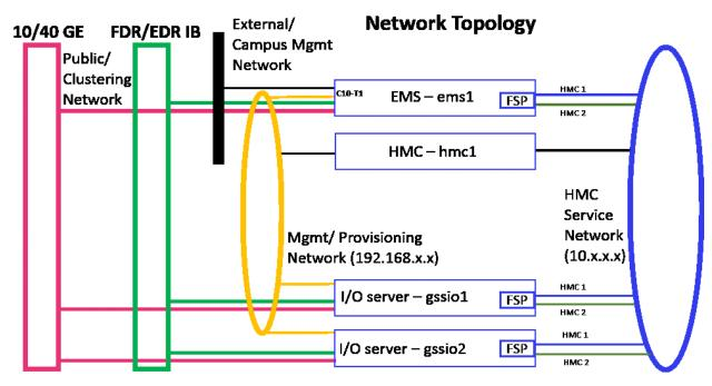
Figure 1. The management and provisioning network and the service network: a logical view (on **PPC64BE**)
