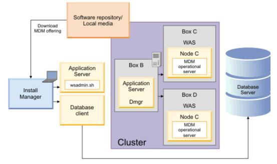
Figure 3. InfoSphere MDM installation in a clustered environment
