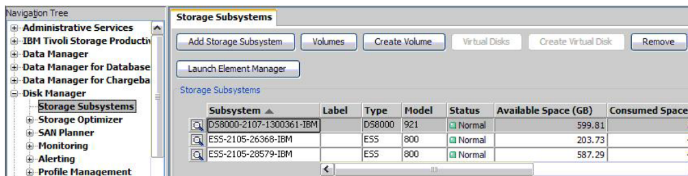
Figure 24. Checking storage subsystems
