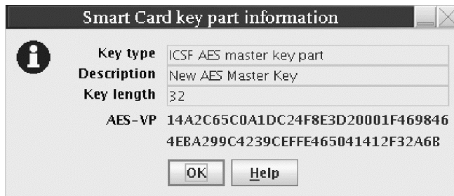
Figure 280. Secure key part entry — AES key part information for a master key
