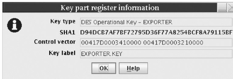
Figure 120. DES Key part register information - add part with SHA-1 for combined key
