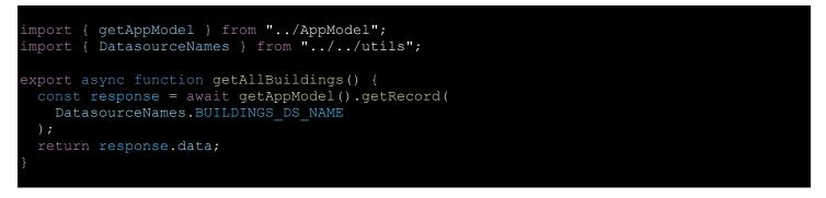
Basically, this code gets the model object and then calls the **getRecord** method to get the data from the **BUILDINGS\_DS\_NAME** data source.
