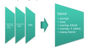
The TRIRIGA team has developed a tool called tri-vulcanize that specifically vulcanizes TRIRIGA UX component files. It pulls the component files from the TRIRIGA server based on the given view to vulcanize, then uses the Google Vulcanize build tool to concatenate these files into a single file
