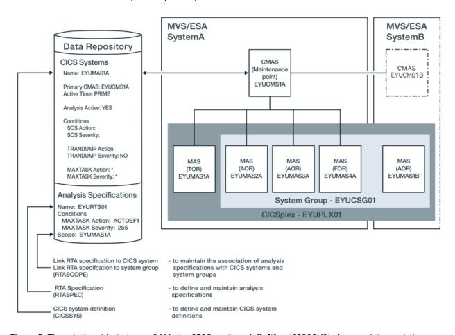
Figure 5. The relationship between SAM, the CICS system definition (CICSSYS) view, and the real-time analysis views
