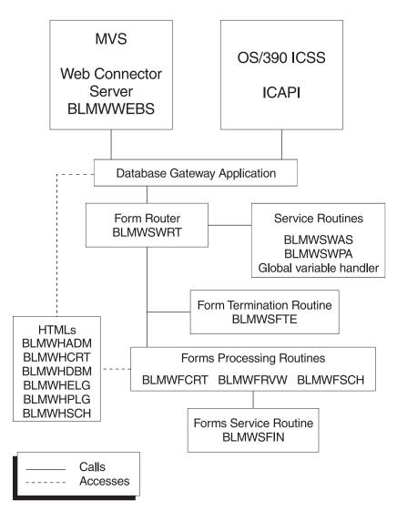
Figure 5. Web connector Interfaces
