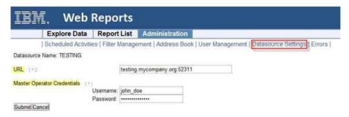
Enter the URL of the root server to which to connect. The URL should also include the appropriate port number.
