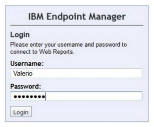
When performing the first log in, the Web Reports uses the Endpoint Manager server to send the login credentials to the LDAP server. If the credentials are accepted, the Web Reports server creates the entry on the database and then logs in the LDAP user.
