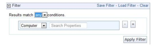
To view a subgroup of the data, pull down the menu to filter by **computer**, **content**, **site** or a previously saved filter. The choice you make determines the secondary fields of the filter. For example, you might want to view computers that have specific operating systems. Click in the box labeled **Search Properties** and enter "OS". There might be a pause while the system collects the properties and verifies the existence of the OS property.
