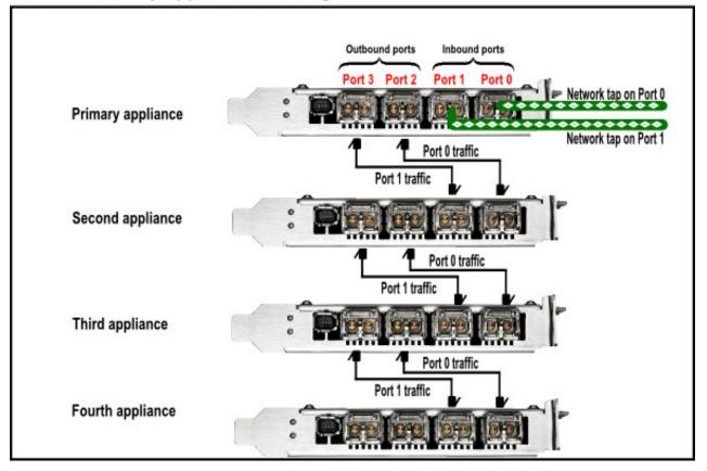
Figure 3. Cabling for stacked 1920 appliances with dual network TAP
