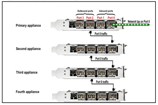
Figure 2. Cabling for stacked 1920 appliances with single network TAP
