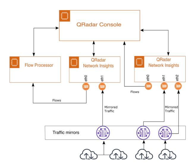
Figure 1. Example of a QRadar Network Insights deployment on Amazon Web Services
