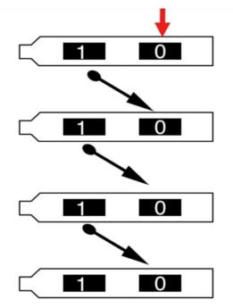
Figure 4. Cabling for stacked QRadar Network Insights 1940 appliances
