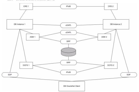
Figure 11-2: Oracle Components and InfiniBand Driver Connections
