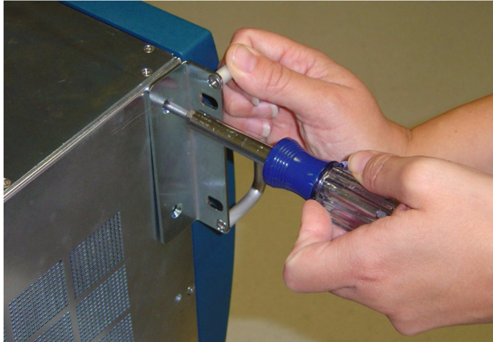
Figure 1-2: Unscrew Extra Mounting Brackets from the Chassis
