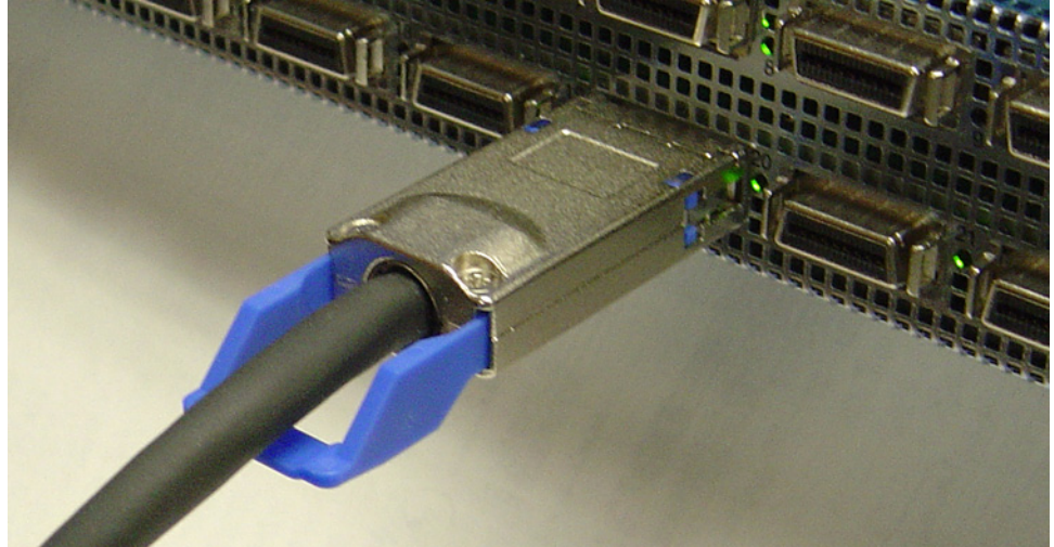
Figure 2-13: Fully Installed IB Cable with Pull Connector
