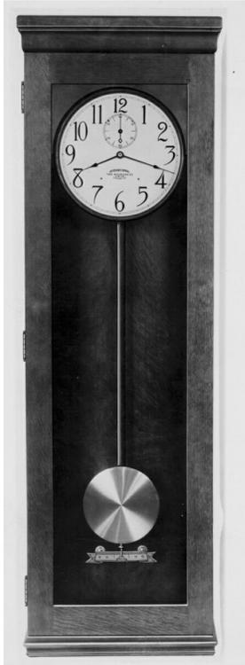
International type B and type C Master Clocks are designed to meet the demand for a medium priced clock that is substantially built and is accurate in operation. These clocks are spring driven and automatically keep themselves wound from a battery, usually the storage battery used to operate the time system controlled by the clock. They wind once a minute and will run for about an hour with the battery disconnected.
