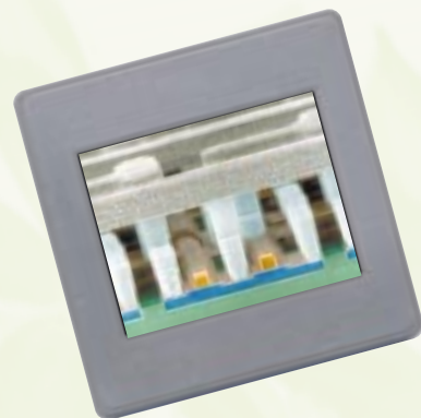
A microscopic image of IBM's Silicon-on-Insulator (SOI) technology. SOI technology results in faster computer chips that require 1.7 to 3 times less power than the older bulk CMOS chip technology.
