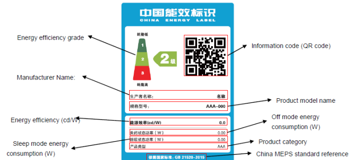
Figure 8. Example of a China Energy Efficiency Label for Computer Monitors
