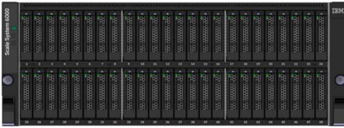
Figure 3. IBM Storage Scale System 6000 is a hardware appliance that allows you to deploy IBM Storage Scale on thousands of nodes with TB/s performance, low latency, and up to 28 million IOPS and 340 GB/s throughput in NVMe deployments.
