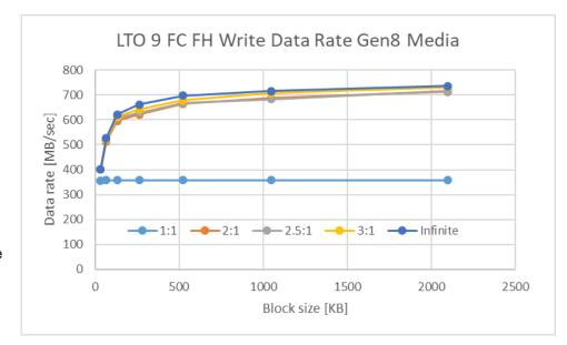
The LTO 9 drive can read and write LTO gen 8 media at the LTO generation 8 operating point. With non-compressible data, a data rate of 360 MB/s is achieved.
