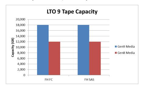
The LTO 9 tape drive with gen 9 media offers a significant capacity increase over gen 8 media.
