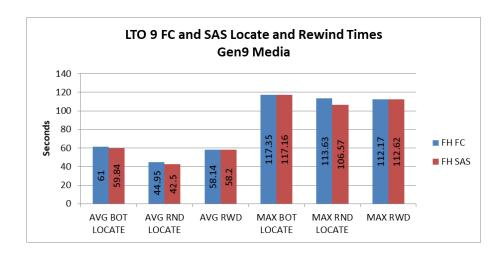
The LTO 9 tape drive with Gen 9 media offers similar performance for Locate and Rewind as compared with Gen 8.
