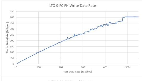
Speed matching helps to improve the overall tape drive data rate at lower host data rates.
