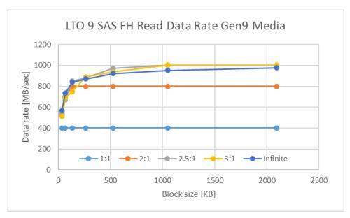
The following charts show the LTO 9 SAS full height tape drive performance when writing or reading LTO gen8 media with data that compresses uniformly at ratios 1:1, 2:1, 2:5:1, 3:1 and maximum (80:1) using differing block sizes.
