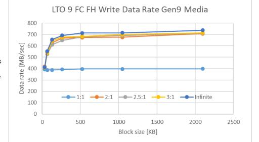
The IBM LTO 9 tape drive achieves a native data rate of 400 MB/s with LTO Gen 9 media. Higher rates are reached with compressible data. LTO 9 uses the same compression engine as LTO 8.
