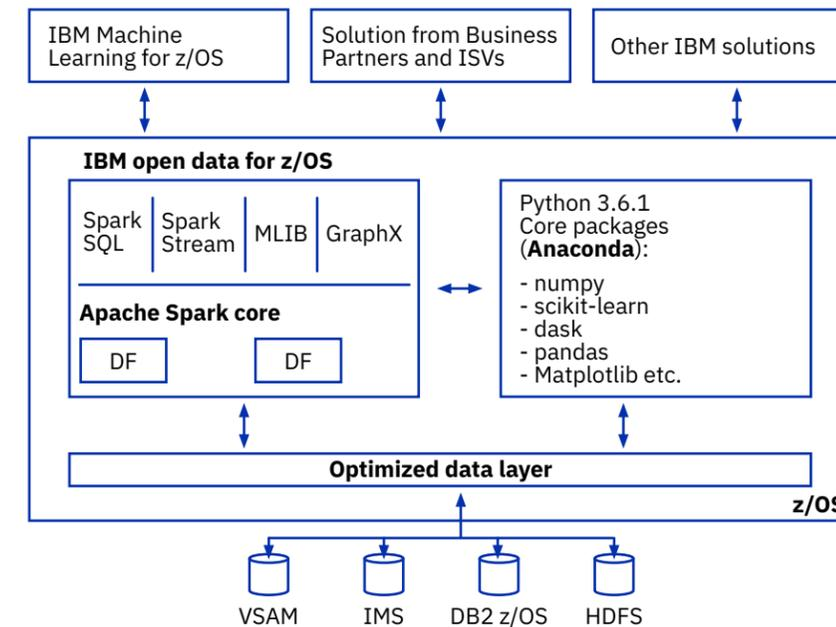
Figure 5: IBM Open Data Analytics for z/OS.
