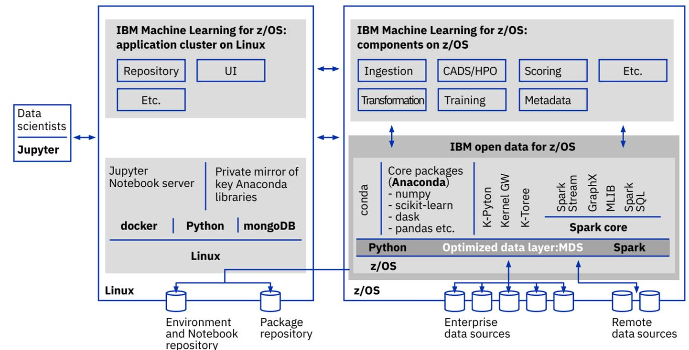
Figure 4: IBM Machine Learning for z/OS Architecture
