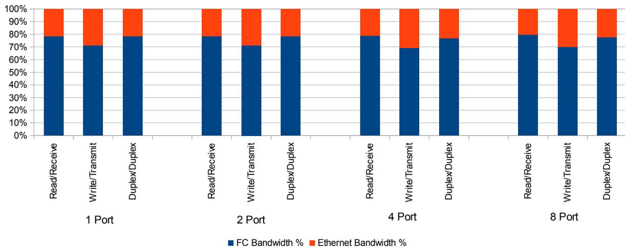
**Fig 10: FCoE and Ethernet Bandwidth Proportionality for Case 2**
