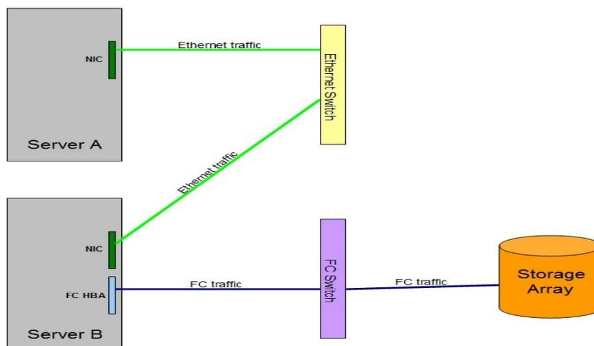
**Fig 1: Traditional setup with FC HBA + Ethernet NIC on a server**
