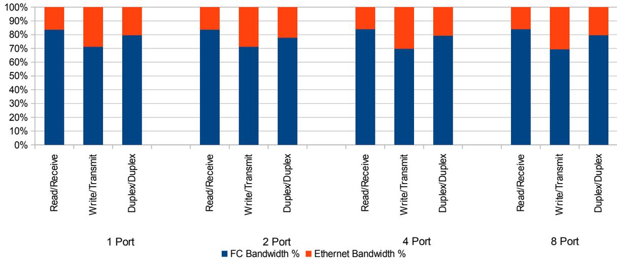
**Fig 9: FCoE and Ethernet Bandwidth Proportionality for Case 1**
