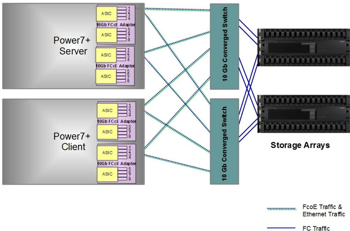
**Fig 3: Test setup with 10Gb FCoE Converged Network Adapter**
