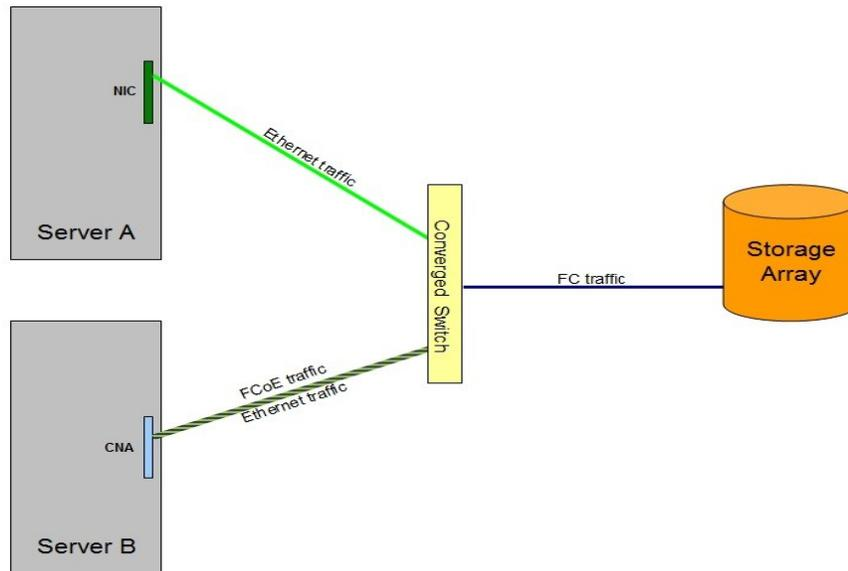
**Fig 2: FCoE CNA on the server used for both FC and Ethernet Traffic**
