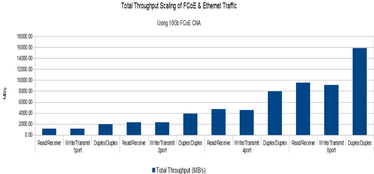
**Fig 8: Total Throughput Scaling of FCoE and Ethernet Traffic**
