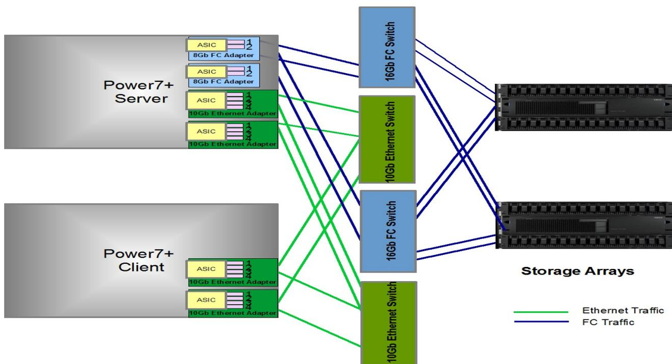
**Fig 4: Test setup with 10Gb Ethernet Adapter and 8Gb FC Adapter**
