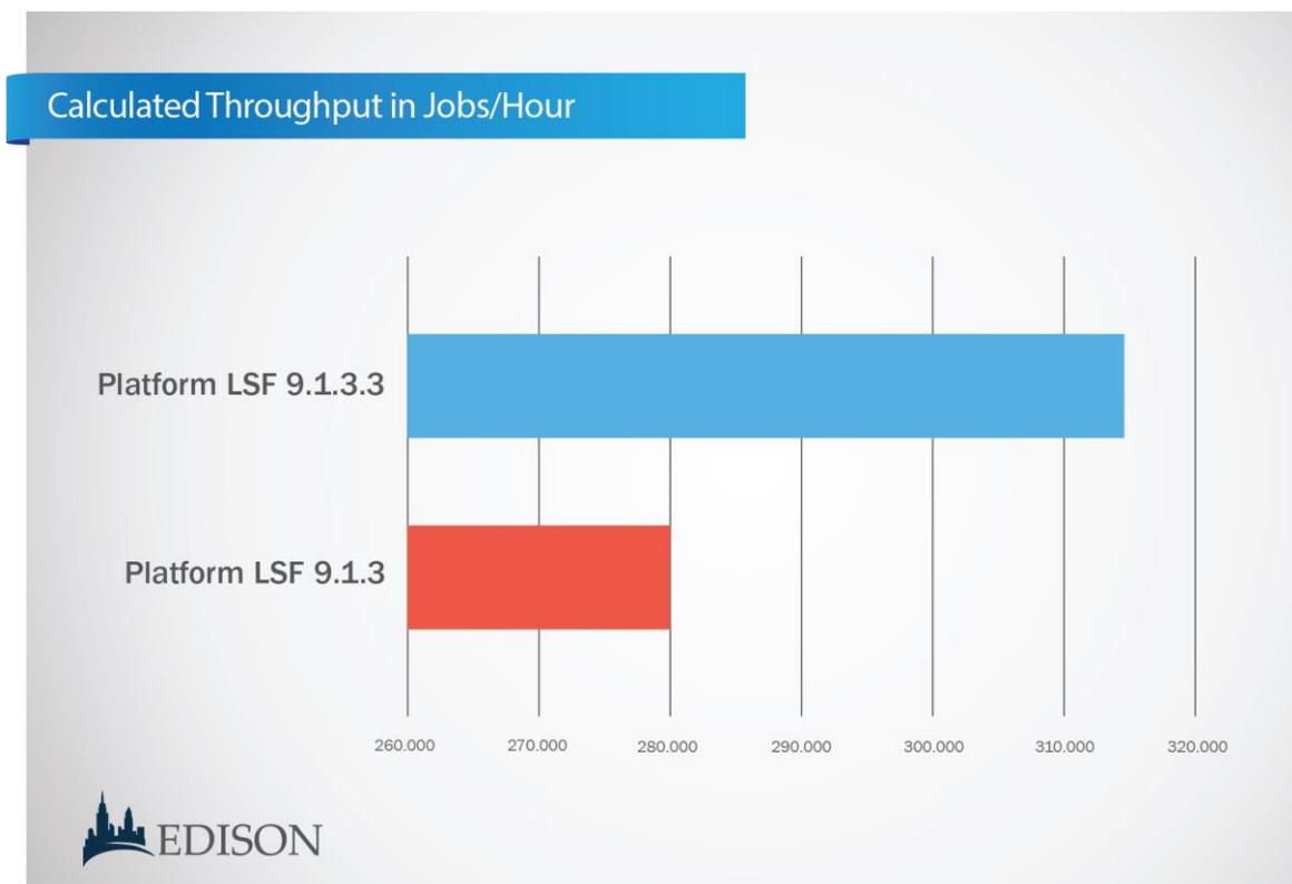
**Figure Three A: Code and Processor Optimization – Real Client Workload Throughput in Jobs/Hour; Platform LSF 9.1.3 versus 9.1.3.3**
