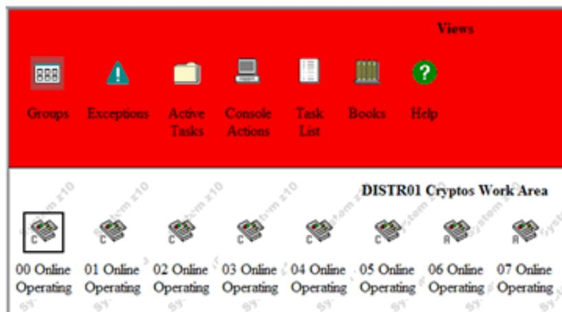
Images Work Area, select the LPAR's image icon, right-click, and select 'Cryptos' to view the status of the AP's assigned to the LPAR:
