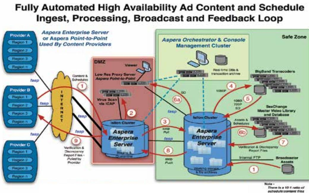
Figure 7: Simplified workflow representations under Aspera Orchestrator control
