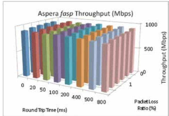
Figure 4: Throughput achieved under various packet loss and network latency conditions on a 1 Gbps link
