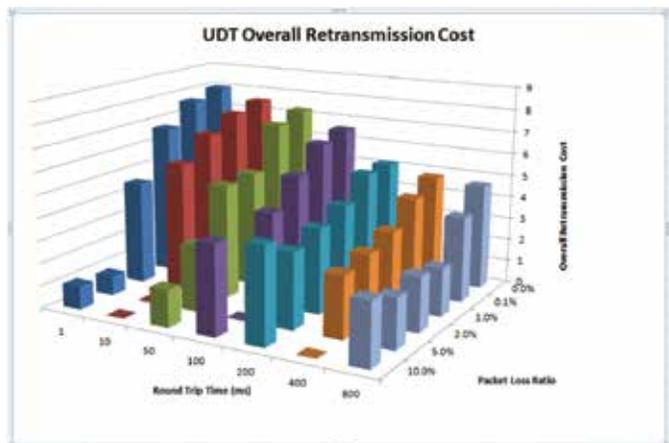
Figure 1: Shows the overall cost of transmitting one packet by a single UDT transfer on a T3 (45 Mbps) link under different RTTs and packet loss ratios. For most typical wide area networks, one packet transfer needs eight to ten retransmissions!
