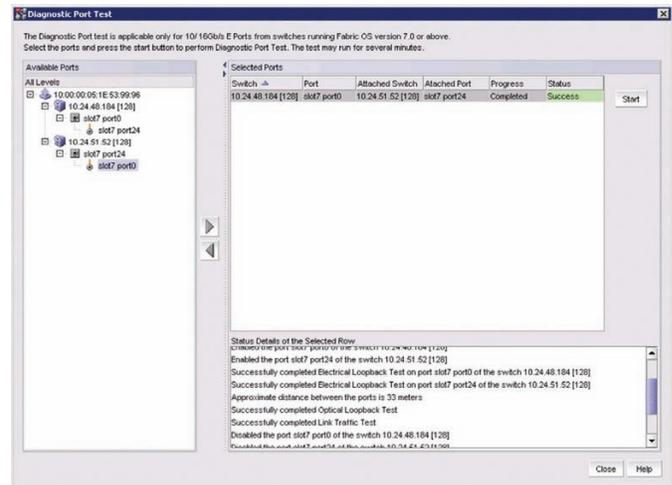
ClearLink diagnostics testing allows storage administrators to run multiple D\_Port tests concurrently to accelerate troubleshooting.
