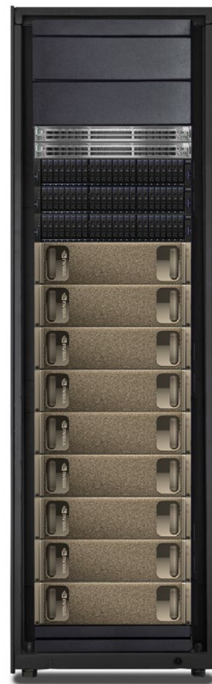
Figure 2: IBM Spectrum Storage for AI with DGX-1 POD, 9:3 configuration
