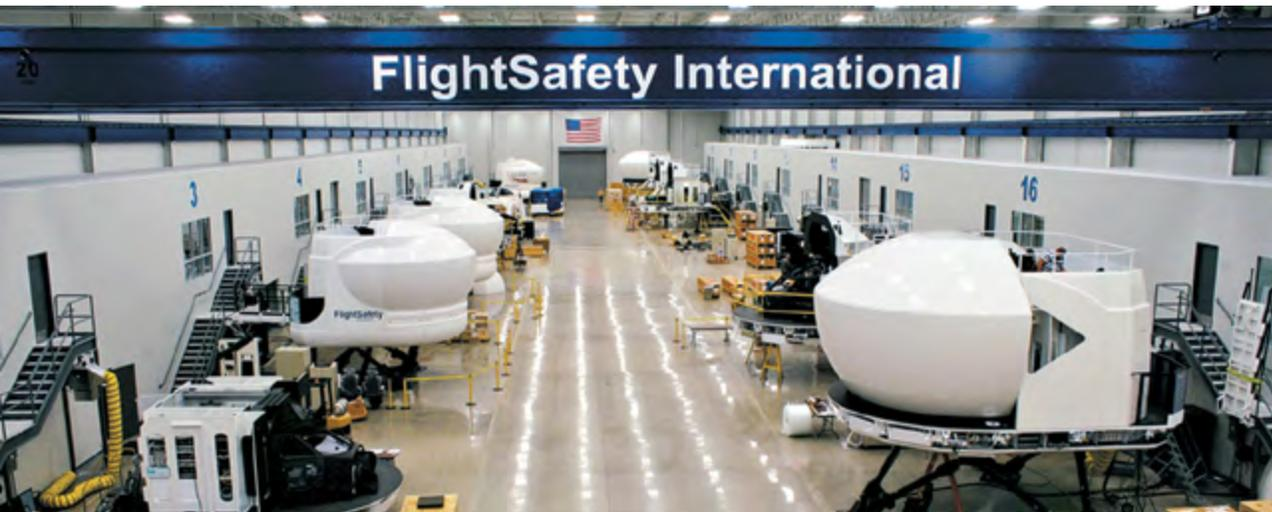
Full flight simulators are large systems—for comparison, roughly the size of a work truck. The interior replicates a full-scale cockpit, with sensors, gauges and backlit screens. These devices cost millions of dollars to engineer and manufacture. To mimic an authentic flight experience, simulators such as the FlightSafety FS1000 are equipped with advanced audio, visual and full-motion capabilities.
