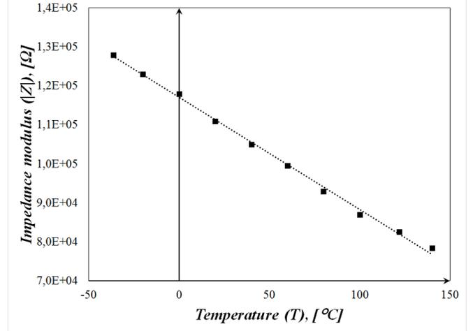
Figure 12: Impedance modulus measured at 1 kHz of the patch sensor as a function of the temperature.
