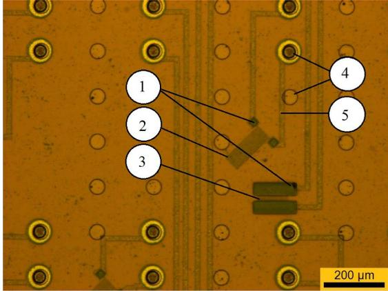
Figure 11: Microscope picture of an integrated sensor at the final step. (1) contact pads in titanium, (2) meander, (3) patch, (4) examples of BLM openings in polyimide and (5) aluminium connection.
