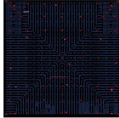
Figure 9: Sensors placement on the chip in order to get for each emplacement (T, RH,  $\epsilon$ ).
