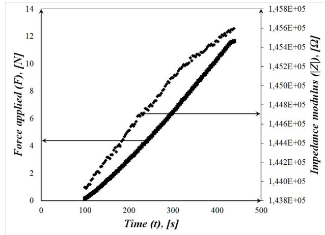
Figure 8: Graphics showing the force applied as a function of time and the impedance modulus measured at 10 kHz of a meander sensor.
