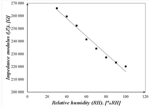
Figure 13: Impedance modulus measured at 1 kHz of the meander sensor as a function of the relative humidity.
