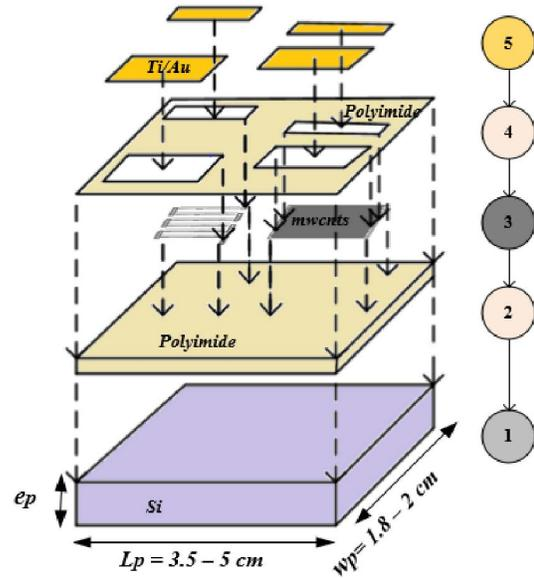
Figure 2: Integration process flow showing the principal fabrication steps of the sensors prototype.
