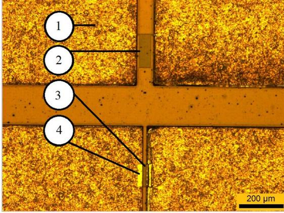
Figure 3: Optical microscope picture of the fabricated prototype. (1) is the electrode, (2) the meander part of the sensor, (3) the patch part of the sensor, (4) the connection area between carbon nanotubes and contact electrode.
