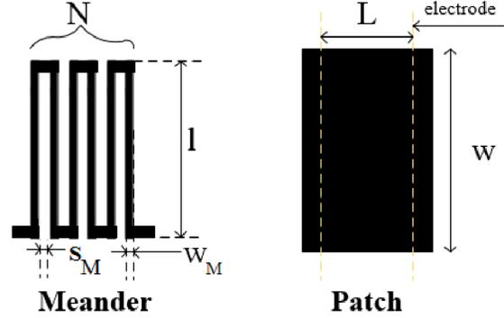
Figure 1: Sensors geometries and parameters definition.
