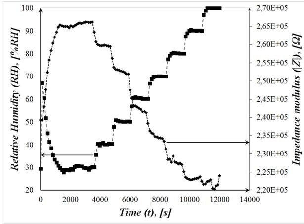
Figure 5: Graphics showing the relative humidity applied as a function of time and the impedance modulus at 1 kHz of a meander sensor.
