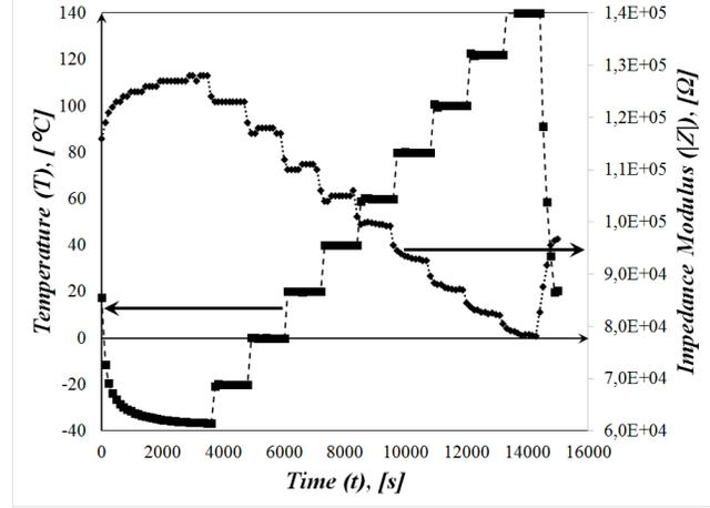
Figure 4: Graphics showing the temperature applied as a function of time and the impedance modulus measured at 1 kHz of a patch sensor.
