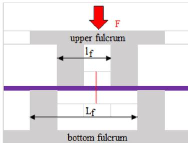
Figure 7: Schematic of the four-point bend test.  $L$  distance between the two bottom fulcrums,  $l$  distance between the two top fulcrums.
