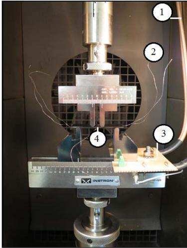
Figure 6: Picture of the four-point bend test. (1) coaxial cables, (2) sensor's wires, (3) test board, (4) prototype.
