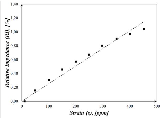
Figure 14: Relative change in impedance modulus measured at 2 kHz of the meander sensor as a function of the strain.
