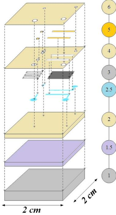
Figure 10: Schematic showing the steps of the sensors within the test vehicle.
