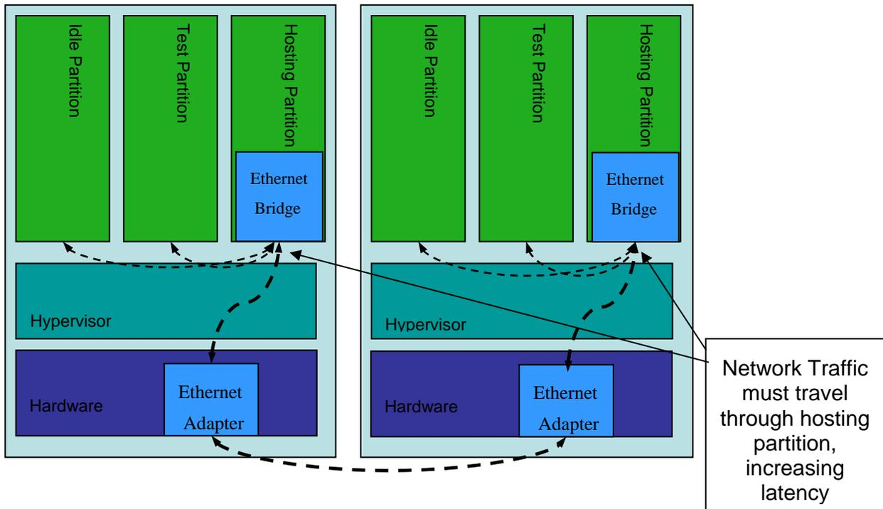
**X86 Systems with four 4 cores and Shared Ethernet**
