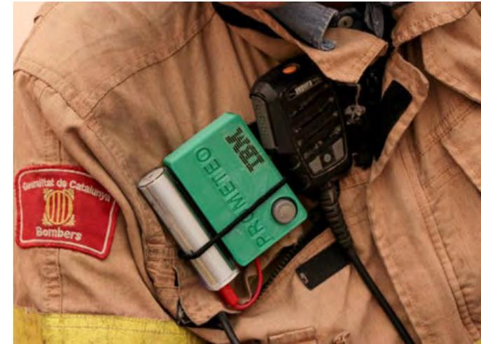
worn by firefighters, who can log in to the device securely with the [IBM Cloud App ID](#) via Bluetooth.
