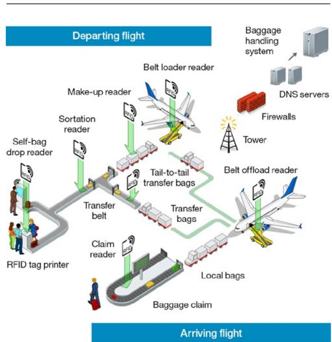
Figure 1: Illustration of the various RFID touchpoints in an airline's baggage operation
