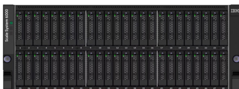
Figure 2 – The IBM Storage Scale System 6000 delivers up to 340 GB/s throughput, 28 million IOPS, and up to 2.2 PB of raw capacity in a compact 4U rack.
